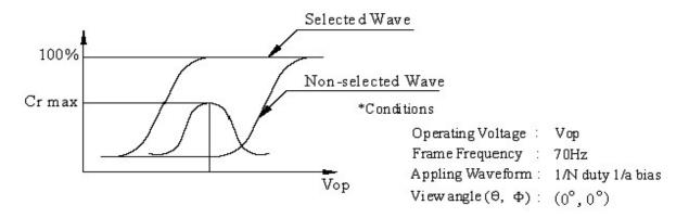
$$Contrast \ ratio(Cr) = \frac{Brightness \ of \ selected \ dots}{Brightness \ of \ non-selected \ dots}$$
