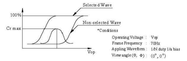
$$Contrast \ ratio(Cr) = \frac{Brightness \ of \ selected \ dots}{Brightness \ of \ non-selected \ dots}$$
